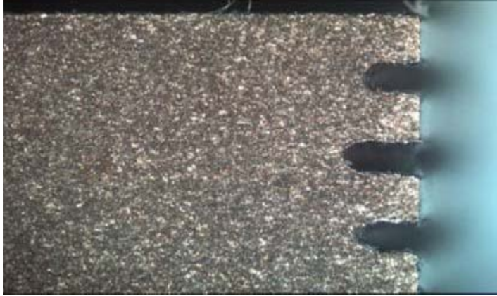
Fig.3. Wire broken and small cutting line in Titanium machining due to low flushing pressure
